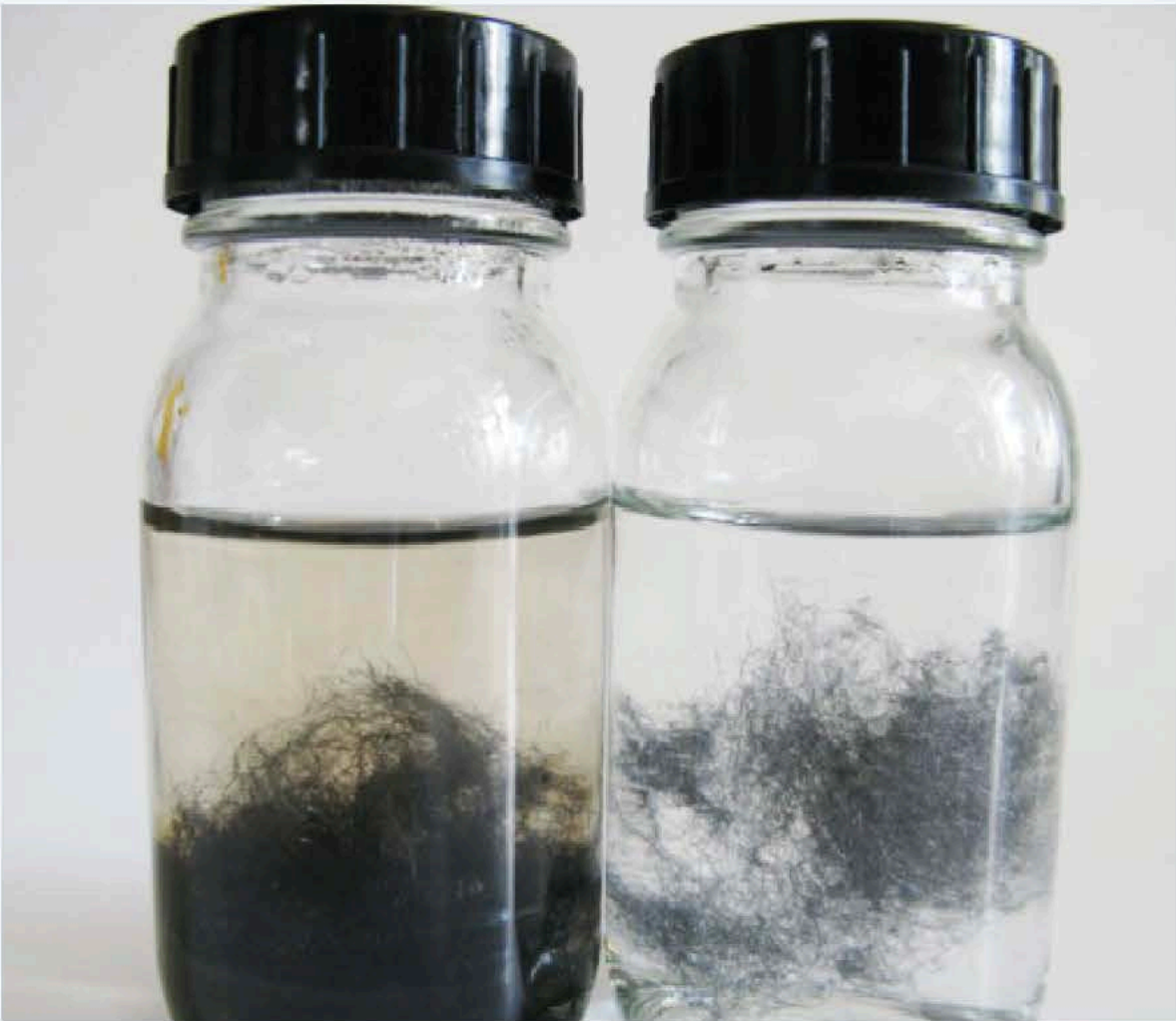
Steel wool in water without (left) and with 2% of WorléeAdd 456 after 48 hours at room temperature
